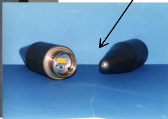
Laser point permanently inserted into guide pin
