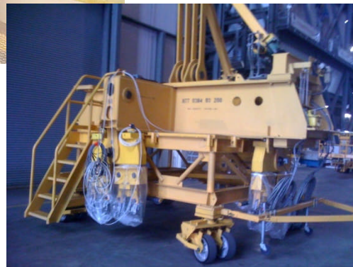
FWD Shaping Beam
